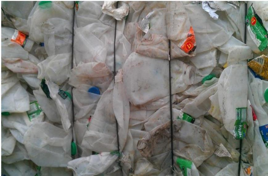
Figure 2 Mixed plastic bale held with horizontal and vertical wires
