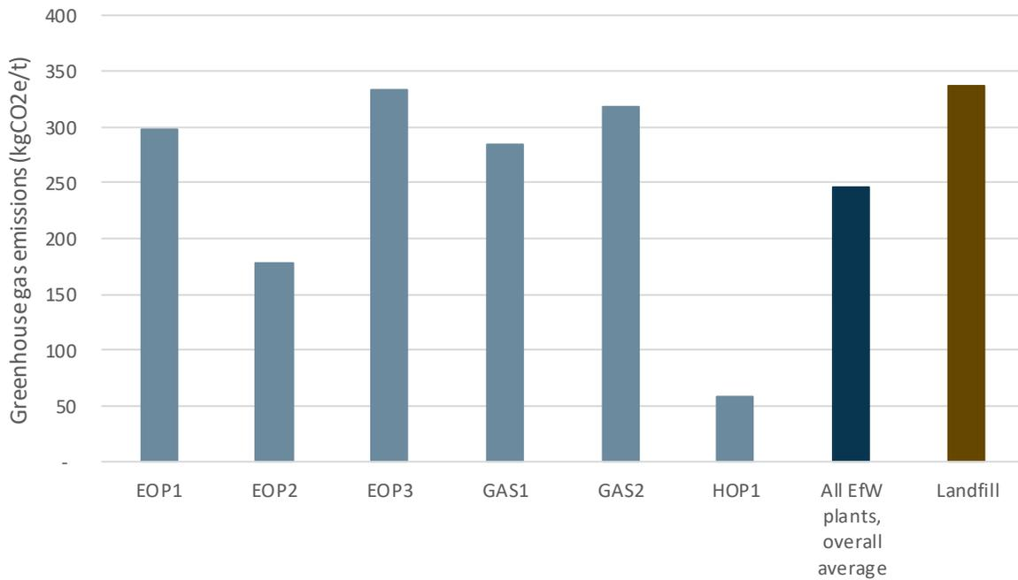
The heat-only plant has lower greenhouse gas emissions per tonne than the other plants because heat-only plants run at a higher efficiency. This means much more energy generation can be displaced by this plant – reducing the greenhouse gas emissions overall.
