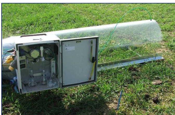
Photo 1: View inside a wind tunnel control box showing the orthophosphoric acid 'bubblers' used to capture ammonia
