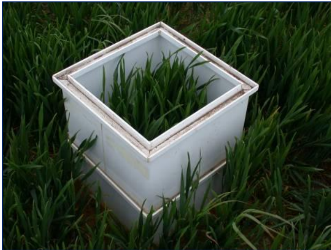
Photo 2. Static chamber used to capture nitrous oxide, methane and carbon dioxide emissions following organic materials applications
